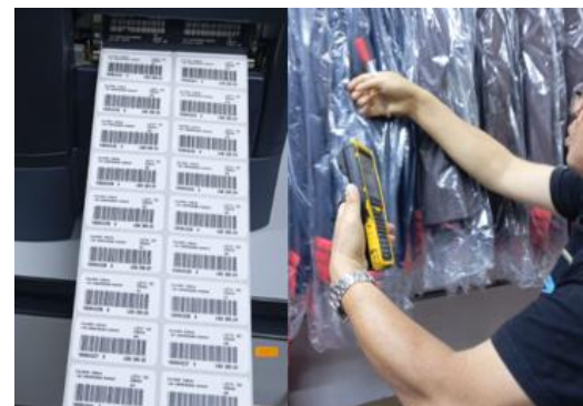
Fig. 2 Use of RFID tags and reader equipment
