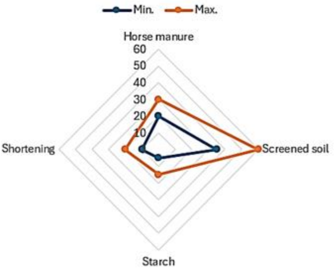
Fig. 6: Percentages of optimal ingredients for the ecological tile material
