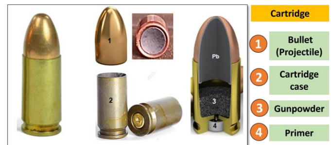
Fig. 2 Ammunition components.
