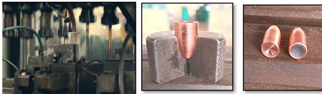
Fig. 14 Lead-free bullet forming machine equipped with a single die
