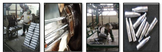
Fig. 11 Lead core casting and forming process
