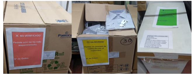
Fig. 5 Packaging Inspection Tracking Cards
