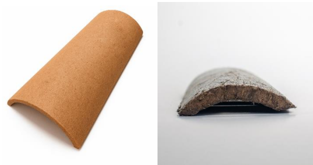
Fig. 5: Mold (right) and shape retention of the tile during the post-molding stage (left)
