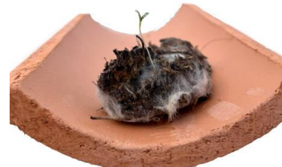
Fig. 7: Ecological tile material undergoing degradation after fulfilling its primary function
