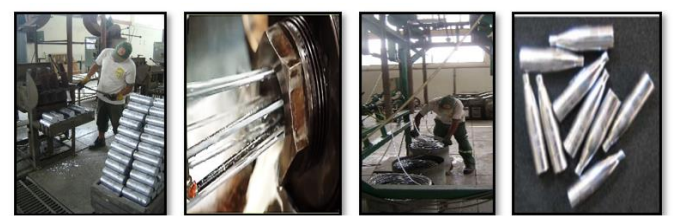
Fig. 11 Lead core casting and forming process
