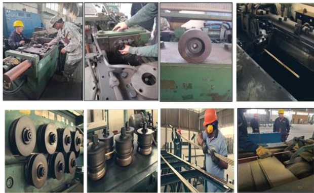
Fig. 7 Combined drawing machine and reducing die
