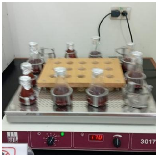
Fig. 6 EDS Copper and cadmium removal tests using grape pomace waste.
