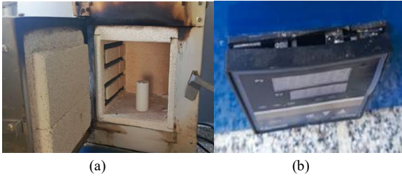
Fig. 3. Mechanical structure (a) Inside the furnace, (b) Damaged components
