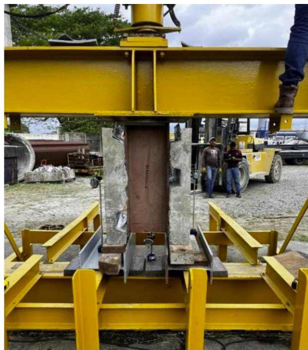
Fig. 5. Push-out test setup using hydraulic press
