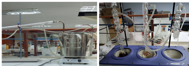
Fig 4. From Left to Right; Molasses distillation setup and Reflux system for accelerated aging simulation.
