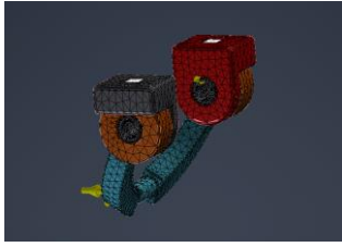
Fig. 5. Malla gruesa generada en Inventor Professional 2026 (Average Element Size = 0.20).
