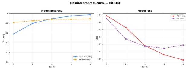
Fig. 21 Training progress curves of the Bi-LSTM model over 5 epochs: accuracy (left) and loss (right) for training and validation sets.
