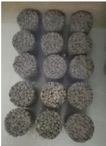
Fig. 1 Permeable concrete samples during curing.
