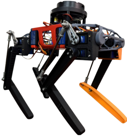
Fig. 10. Fully assembled quadruped inspection platform used in the hardware-in-the-loop validation campaign.
