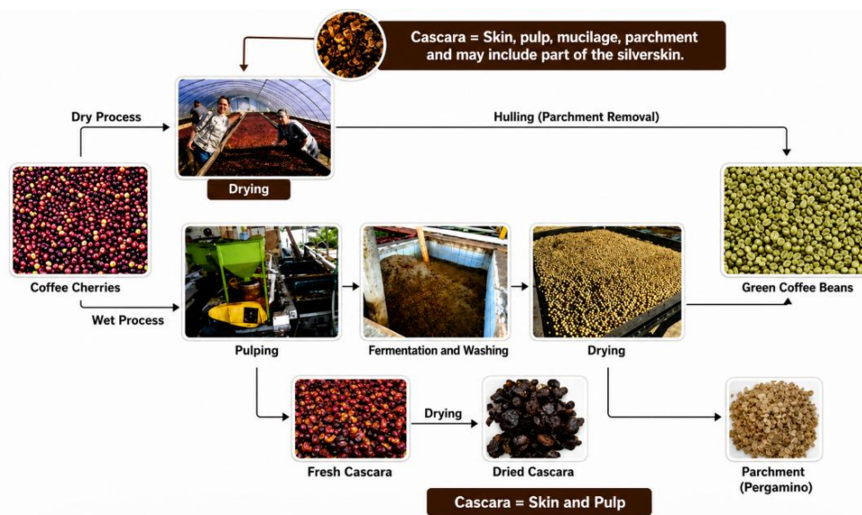
Fig. 2 Coffee processing stages illustrating dry and wet processing routes and the generation of pulp and husk residues used as raw material..
