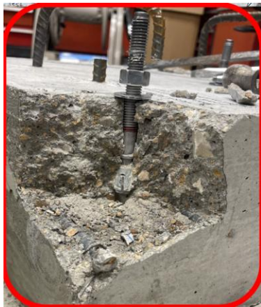
Fig. 7 Modes of failure of Mechanical Anchors Hilti KB-TZ2 \frac{1}{2} " \phi – 3 \frac{3}{4} " embedment
