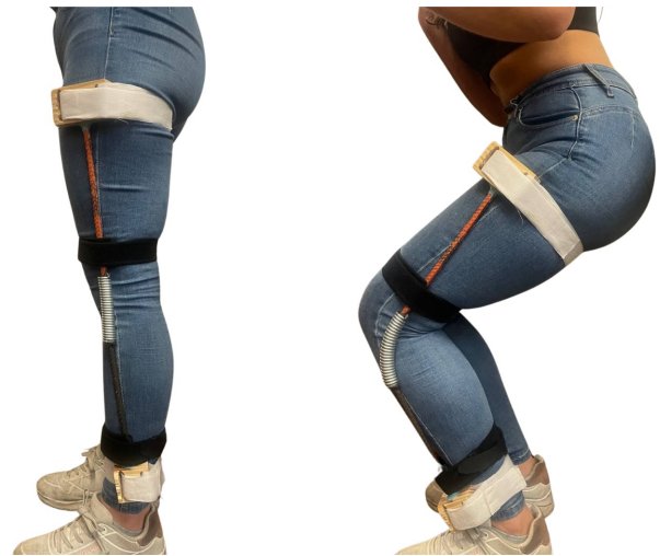
Fig. 2. Final prototype iteration of the passive wearable device assembled with low-cost materials and Velcro-based fastening.
