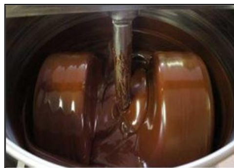
Fig. 5. Refining and conching.
