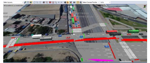
Fig. 7. Functional geometric redesign of the intersection – Case 2.
