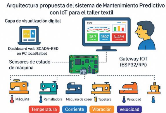
Fig. 4 Proposed architecture of the PdM system with IoT
