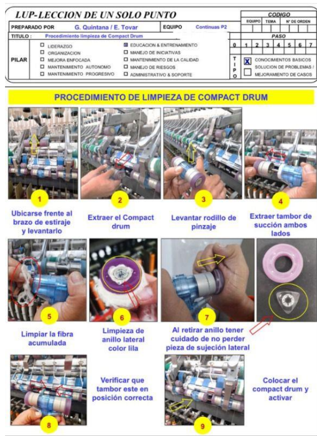
Fig. 3. Standardized Compact Drum Cleaning Procedure (LUP)
