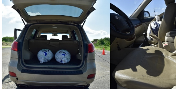
Fig. 3: Loaded condition setup used to represent an increased vehicle mass state.
