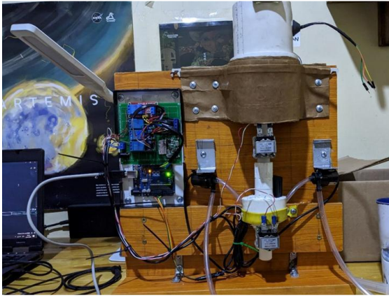
Fig. 3 Physical assembly of the automated precipitation sampling prototype, detailing the collection chamber, hydraulic lines, and distribution valves.
