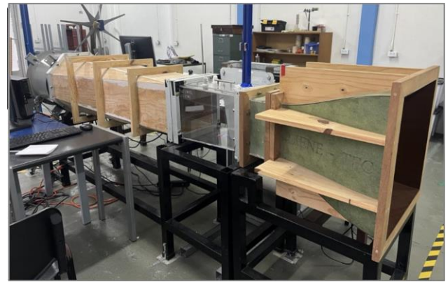
Fig 3. Wind tunnel used to the prototype test.
