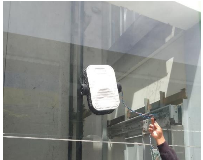
Fig. 18 Experimental Validation of the Robot Operating on a Vertical Surface.
