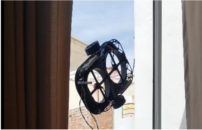
Fig. 17 Static Vertical Adhesion Test Using the Vacuum System.
