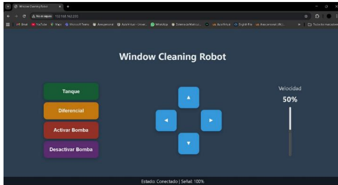
Fig. 15 Web-based control interface deployed and connected through IP address.
