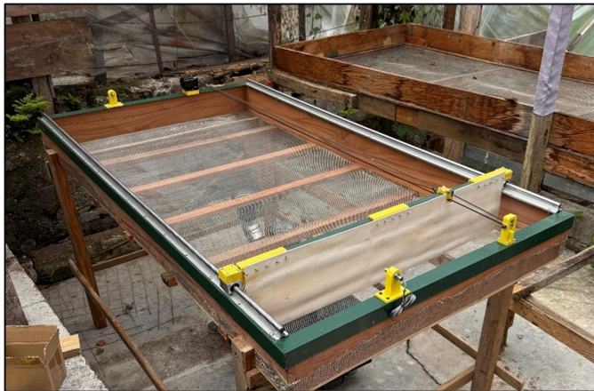
Figure 4: Integrated automated raking and linear motion system.
