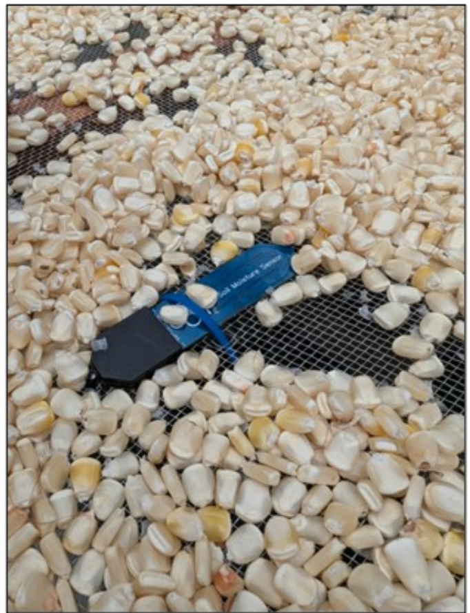
Figure 8: Capacitive sensor used to measure the moisture content of corn kernels
