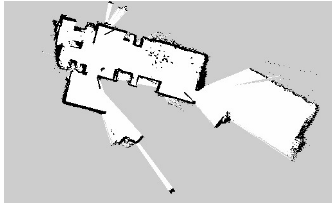
Fig. 2. Occupancy grid map generated by the KARNAV prototype using LiDAR-based SLAM.
