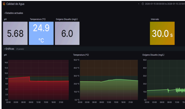
Fig. 8 Dashboard with real-time monitoring of pH, temperature, and DO during the experimental test.
