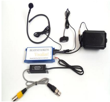
Fig. 1 Bluetooth Mobile Phone Voice Control System for wheelchairs
