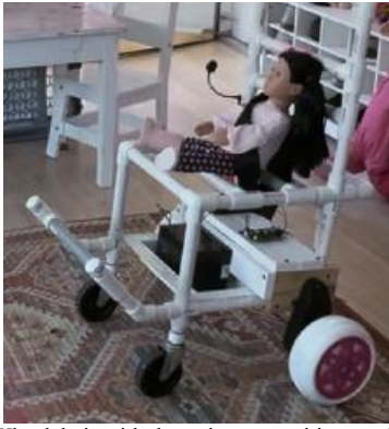
Fig. 8 Wheelchair with the voice recognition module test.
