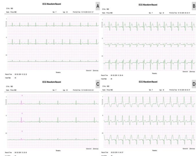
Fig. 4 Pathologies simulated on MECEG 180D device for sensitivity purposes performed with the PS-2200 multi-parameter patient simulator
