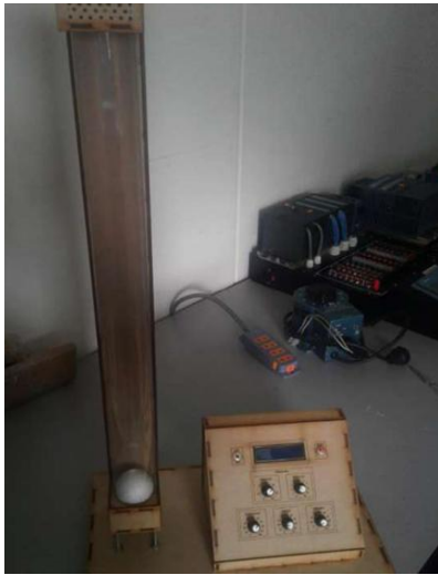
Fig. 7 Pneumatic levitation prototype implemented
