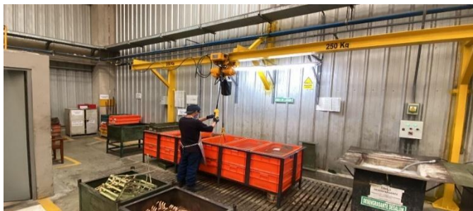
Fig. 9 Semi-automated monorail for chrome plating
