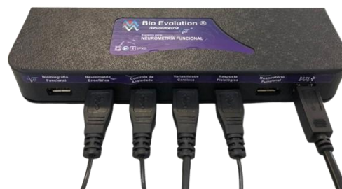
Fig. 2 Cabinet with channels for connecting the sensors
