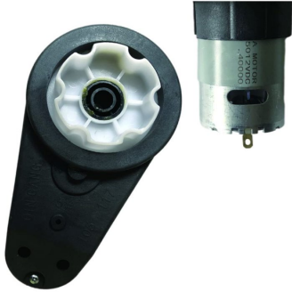
Fig. 3. Gearbox and motor implemented in the Amity Rover. Source: [14].
