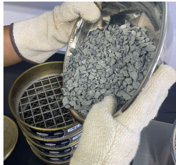
Figure 3. Pouring Basalt Gravel Aggregate into Sieves for Particle Size Analysis
