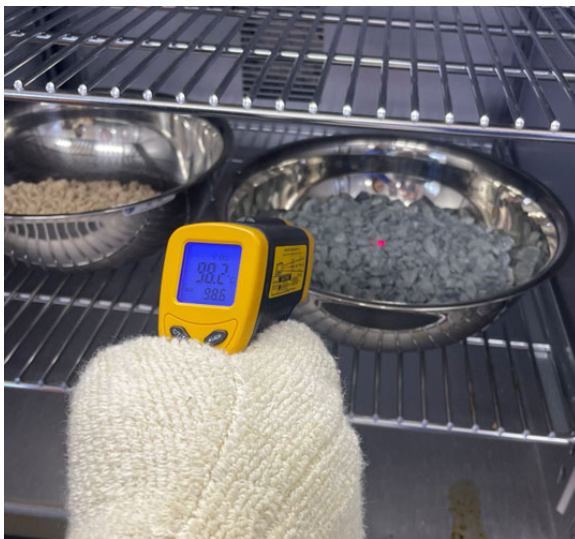
Figure 4. Aggregates in Oven for Drying
