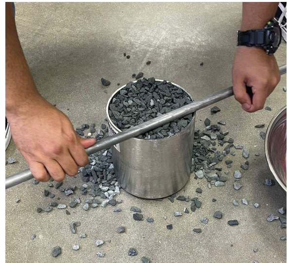
Figure 5. Basalt Gravel being Compacted by Rod in Cylinder Mold for the Bulk Unit Weight Test
