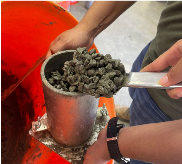
Figure 1. Basalt Gravel Pervious Concrete Molding in Cylinder
