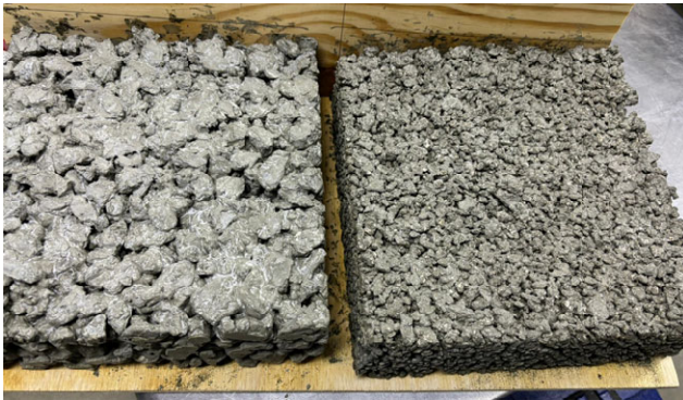
Figure 2. Pervious Concrete Slabs
