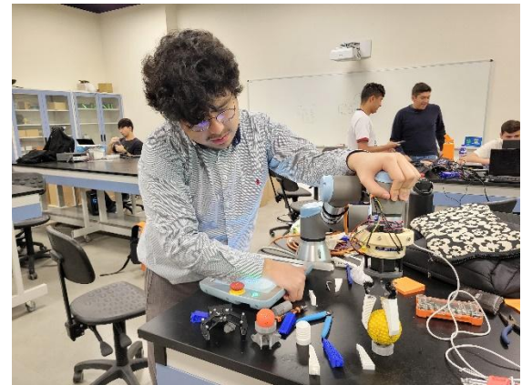
Figure 2. Integration a "soft gripper" with a UR collaborative robot.
