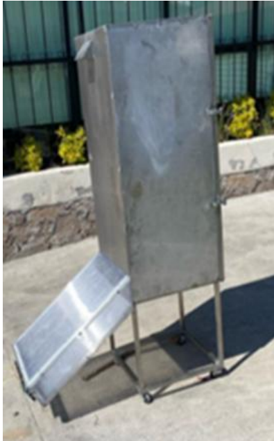
Fig. 2 Solar dehydrator prototype without forced convection.
