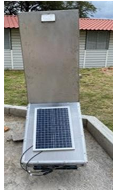
Fig. 3 Solar dehydrator prototype with forced convection.
