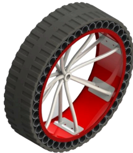
Fig. 1 Wheel design focused on pressure points.
