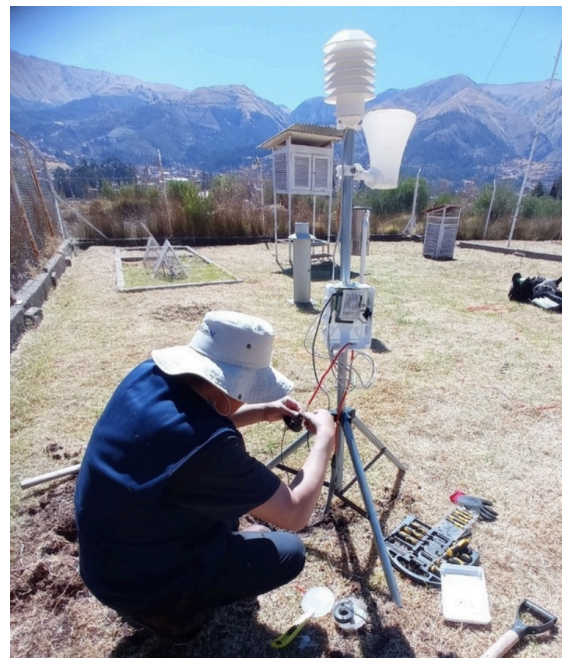
Fig. 2. State of the art 2: Semanhi weather station 3D-printed in PLA, installed in Cusco.
