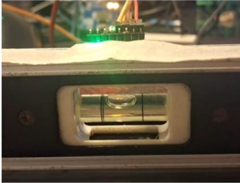
Fig. 10 Sensor compared with a bubble level
