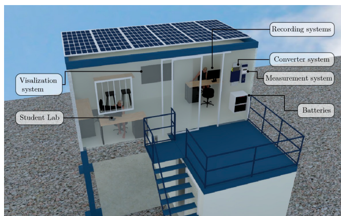
Fig. 4 KIOSOL project with solar panels, hybrid inverter and batteries. Source: An Intelligent Distributed Energy Resources Living Laboratory [16].
