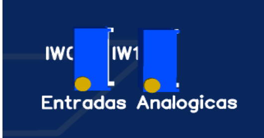
Fig. 9. Analog Inputs with Potentiometers in the Prototype. Source: Authors.
