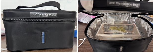
Fig. 1: UV-C system used to irradiate lentil seed in December 2024.
