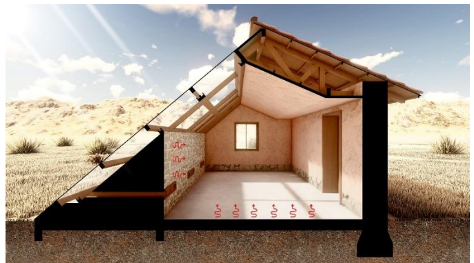
Fig. 2 Passive Collector System Operating as a Direct Collector with Thermal Inertia. The figure shows a passive collector system working as a direct collector based on thermal inertia.
