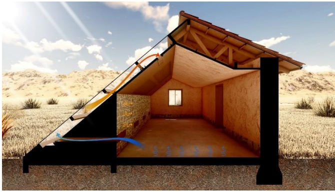
Fig. 3 Passive Collector System Operating as a Collector with Air Convection. The figure shows a passive collector system working as a direct collector based on air convection.
