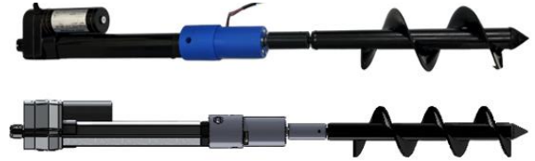
Fig. 4 CAD vs Real Life model of drilling mechanism
