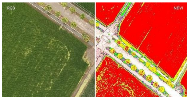
Fig. 5 Images according to camera types and spectra (RGB and NDVI).
