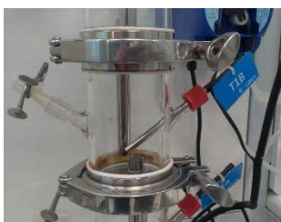
Fig. 4 Temperature sensor of one of the column stages
