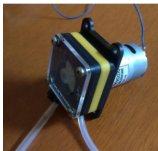
Fig. 9 Peristaltic recycling pump
