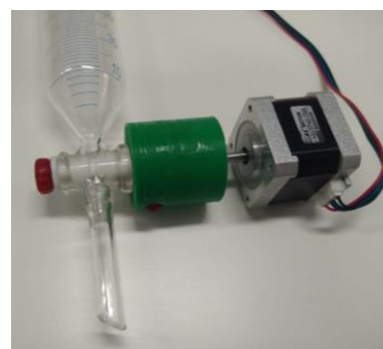
Fig. 7 Stepper motor coupled to the burette valve
