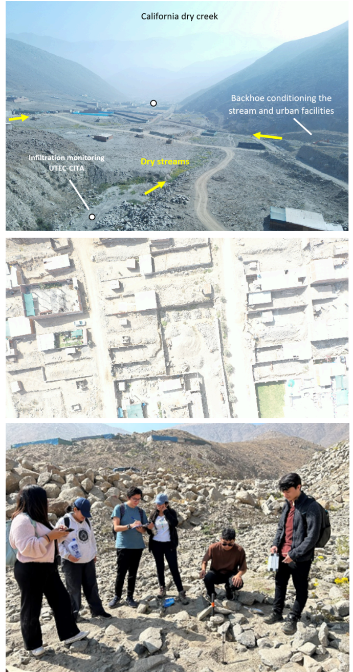
Fig. 2 Panoramic downstream view (top), a plan view of shanty towns configuration (middle) and field work by UTEC students with infiltration tests and soil samples (bottom).
