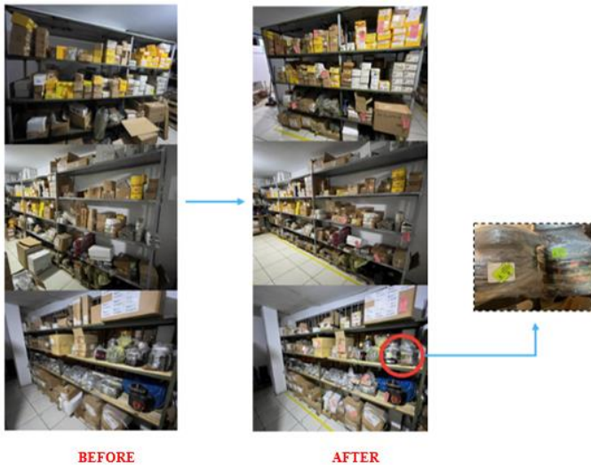
Fig. 8: Implementation of Phase N°02: Seiton (set in order)
