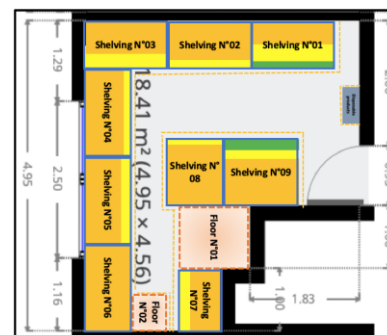
Fig. 5: Layout of warehouse No. 06 by percentage of occupancy (%) according to the ABC categorization of products relocated and stored after the implementation of the Systematic Layout Planning
