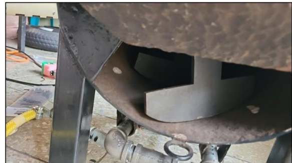
Fig. 11 Mixing shaft and roasting chamber.
